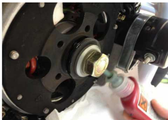
Fig. 4 – Loctite 648 on inner and outer thread
