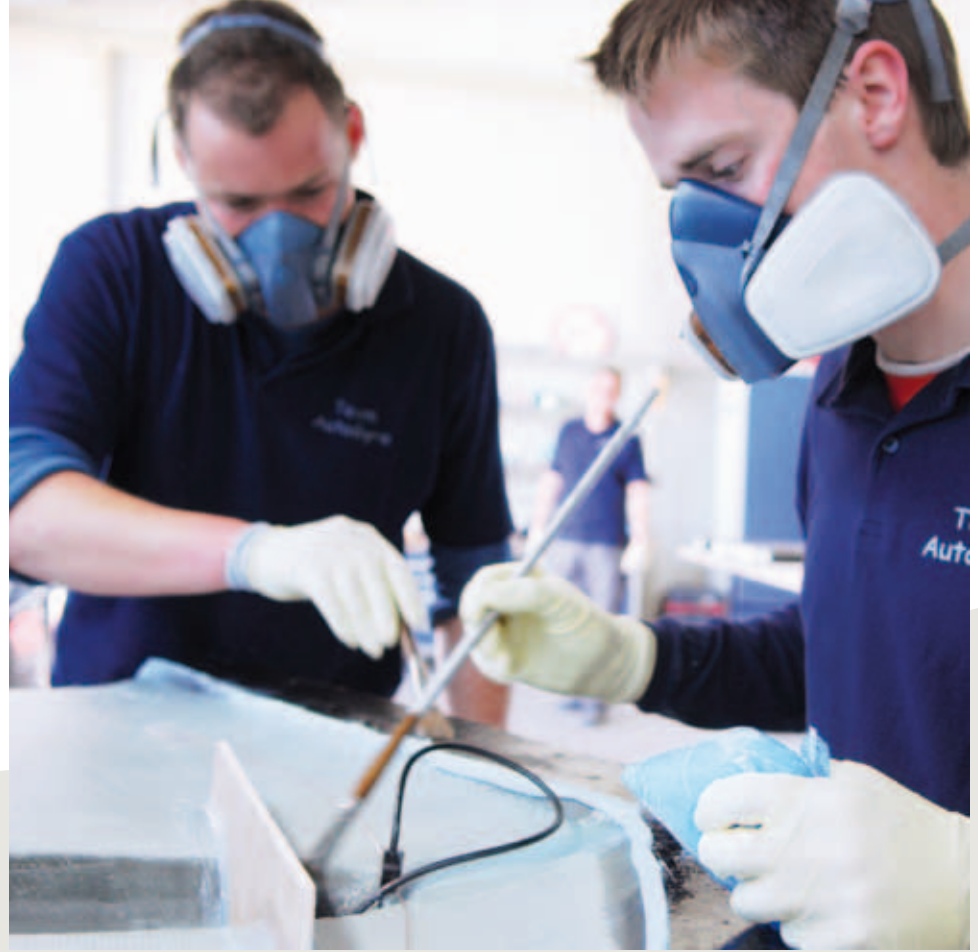
Laminating the reinforced plastic parts
